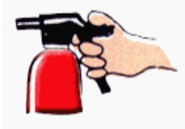
**S**weep from side to side at the base of the fire until extinguished.
